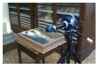
Fig. 1. Structured light scanning survey of a XIX° century costal area plastic model
