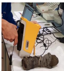
Portable X-ray fluorescence analyses carried out in Mazarrón II.
