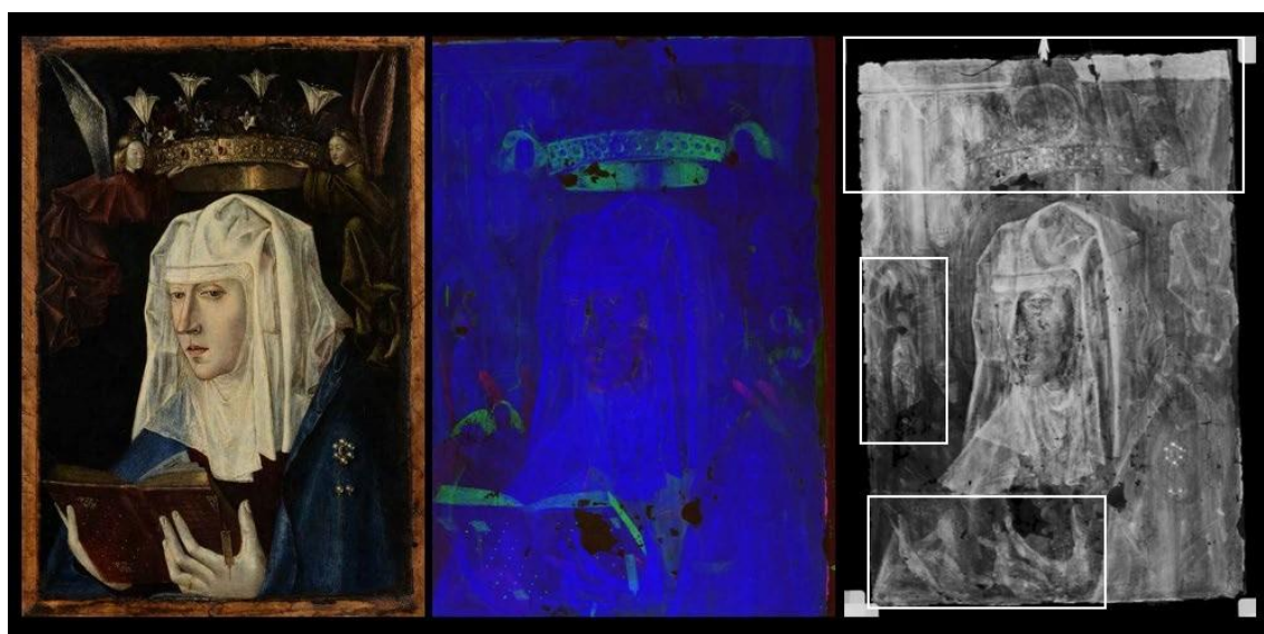
From the left: a) The Reading Virgin , attributed to Antonello da Messina (ca 1430-1479); b) Macro-XRF map of Hg-L (red); Fe-K (green) and Pb-L (blue); c) X-ray radiography.
